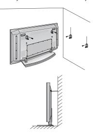
. After the set must be mounted on the desk top, install the TV brackets on the TV as shown.
